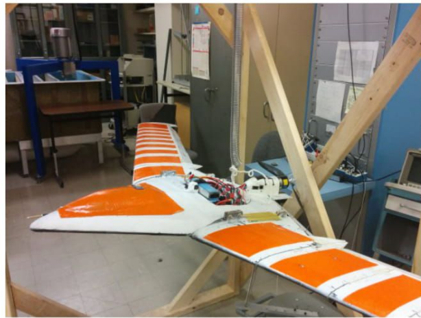
Figure 1: A small flying wing aircraft set up for GVT
